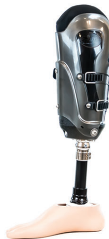
Figure 2. Medial view of iFIT transtibial prosthesis showing the notched hooks that grab the cables that curve around the back of the socket. This allows small adjustments to the circumference of the socket both proximally and distally with the two-buckle system.
