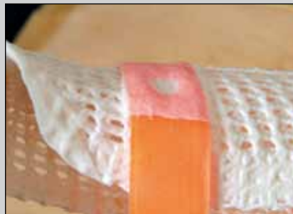
7. Press the strap with the Edging material into the orthosis and let cool.
