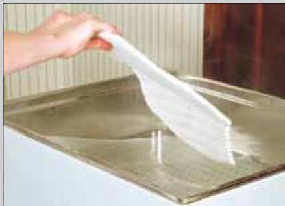
9. Heat edges one by one in water bath.
