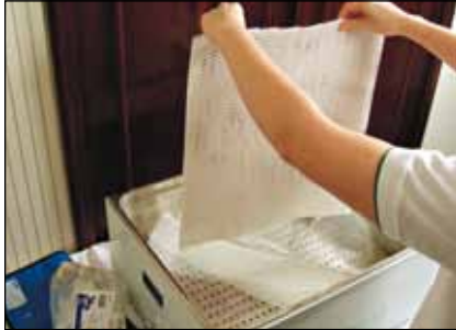
3. Hold the three sheets together and immerse in water for a few seconds to adhere together.
