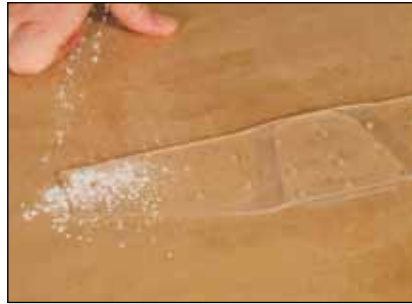
18. Place the foot piece reinforcement onto the stirrup in the heel area. Put talcum powder onto the ends to avoid sticking together.
