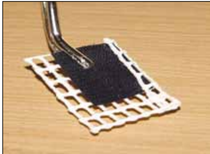
3. Use a heat gun (or immerse to water) and fold up the three edges around the Velcro.
