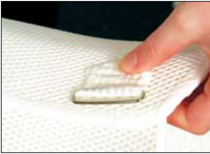
15. Press heated buckles into place. Repeat procedure with remaining buckles
