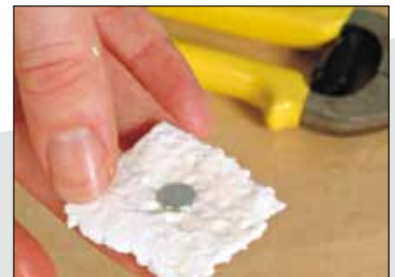
7. First remove the X-LITE® with the T-nut from the water and press the material and the T-nut together firmly.
