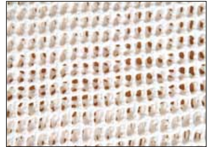
2. Prepare the three sheets of X-lite - the middle sheet should be in the opposite direction for increased rigidity.
