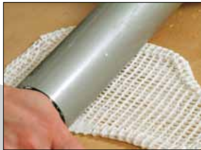
5. Heat edges one by one in water bath. Using a rolling pin compress only the covered edges firmly to create a smooth finish.
