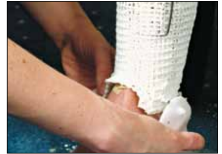
19. Place the foot piece under the foot and bring the stirrup side up. Press the top of the stirrup firmly against the exposed rivets to get a good protruding mould.
