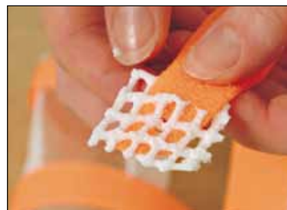
4. Fold the heated X-LITE® material and press firmly together
