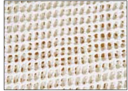
2. Prepare the three sheets of X-LITE® - the middle sheet should be flipped in the opposite direction for increased rigidity.
