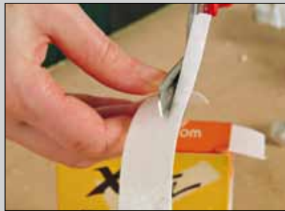
1. Cut X-LITE® Edging Material to desired width and length.
