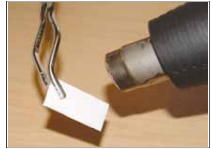
15. Use heat gun to soften the thermoplastic hook (8-10 sec.).
