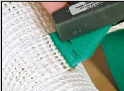
25. Attach the straps to the underlying side, using heavy duty staples or other suitable method.
