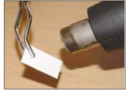
2. Apply dry heat to back side until sticky.
