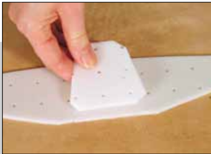
6. Cut the foot piece reinforcement and stirrup from the Aquaplast or similar material.
