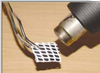
5. Heat the back side with a heat gun until sticky.
