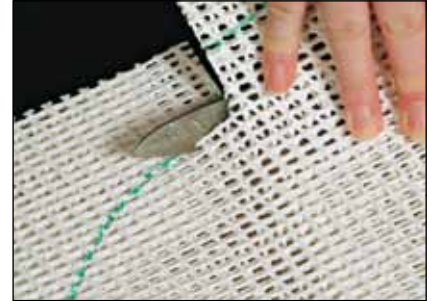
5. Heat areas to cut in water to soften and then cut.
