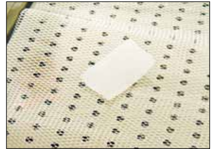
3. Immerse Edging material into water, for a few seconds.
