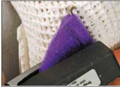
17. Attach the straps to the underlying side, using heavy duty staples or other suitable method.
