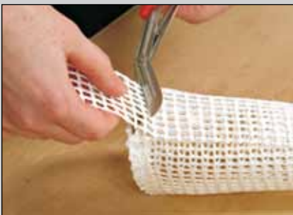
10. Cut re-inforcement to proper length.
