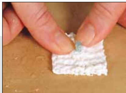
7. First remove the X-LITE® with the T-nut from the water and press the material and the T-nut together firmly.
