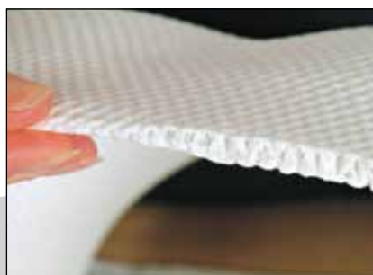
8. Heat small sections of edge in water bath or with heat gun and press edges together.
