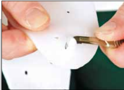
20. When the stirrup has cooled - use a sharp knife to remove the material covering the holes.
